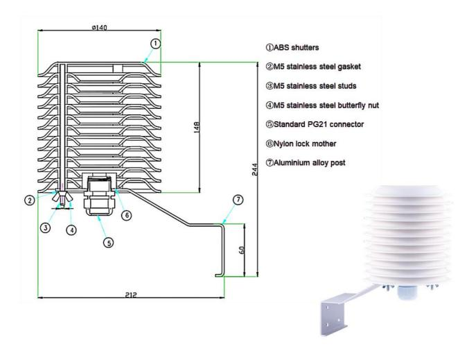
1.Install the product in stable environment area, avoid direct sunlight, away from windows air-conditioning, heating and other equipment. Otherwise it will cause measurement inaccuracies.
