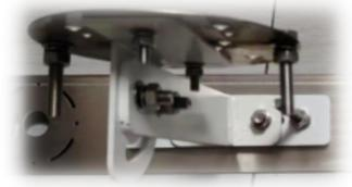
The sensor should be installed in the open air without any cover above the sensing surface.
