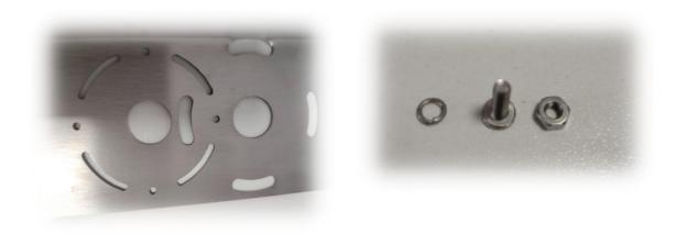
**Step 3:** Align the screw holes on the wind direction sensor with the holes on the mounting support, and lock the screws(4psc). Please make sure the marker is pointed to the **south** during installation(you can use a compass for positioning).
