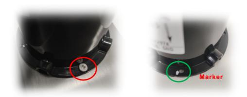
**Step 4:** Connect the navigation connector to the sensor base connector.
