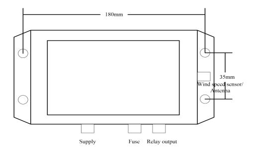
Step 3: Flange mounted, fix four screws on the bracket and keep the product horizontal.
